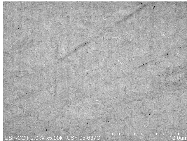
Figure 3.8 Plan-view SEM image shown at a magnification of 5.0k for a representative 3C-SiC layer grown with the HCl process at a rate of ~8.6 \mu\text{m/h} grown. Image courtesy of D. Edwards, USF COT.
